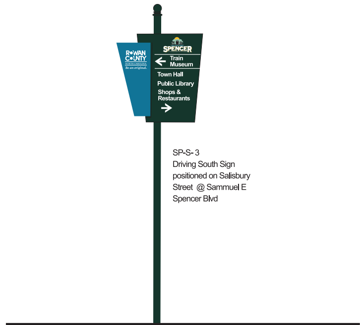
MAIN STREET/PEDESTRIAN WAYFINDING / 3.5" LETTERING FOR SPEEDS BELOW 35 MPH
